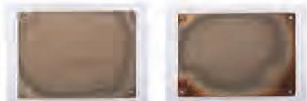
Both of these test panels were exposed to very harsh, salt-water conditions on the coast of Australia. The left panel is an example of AZM brand metal roofing. The right panel is standard galvalume... As you can see corrosion is rapidly creeping in on each corner of the galvalume panel.
